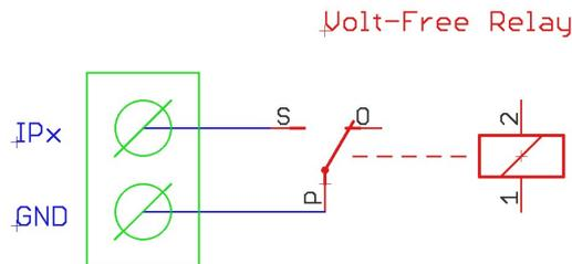
Setting the input to digital will overwrite the upper and lower threshold voltages to 20V and 10V respectively. The source voltage will be 2.8V maximum.
