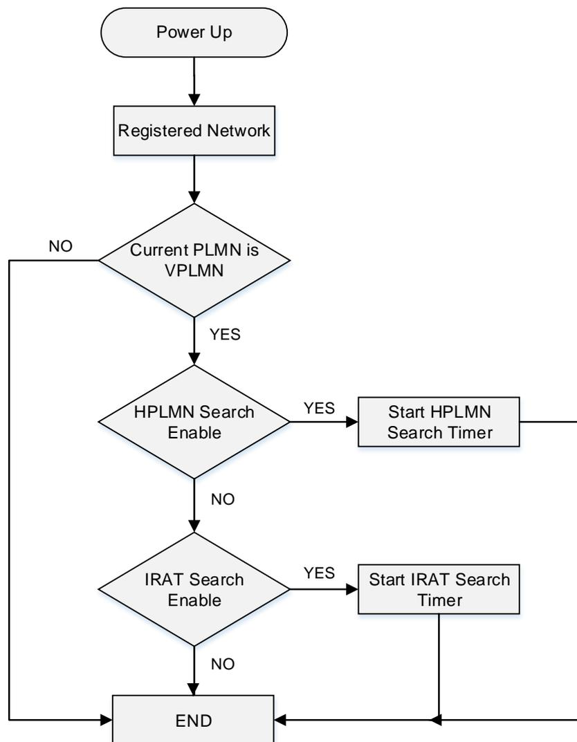
Figure 5: Behaviour of the Module if (U)SIM is Card in Roaming State
