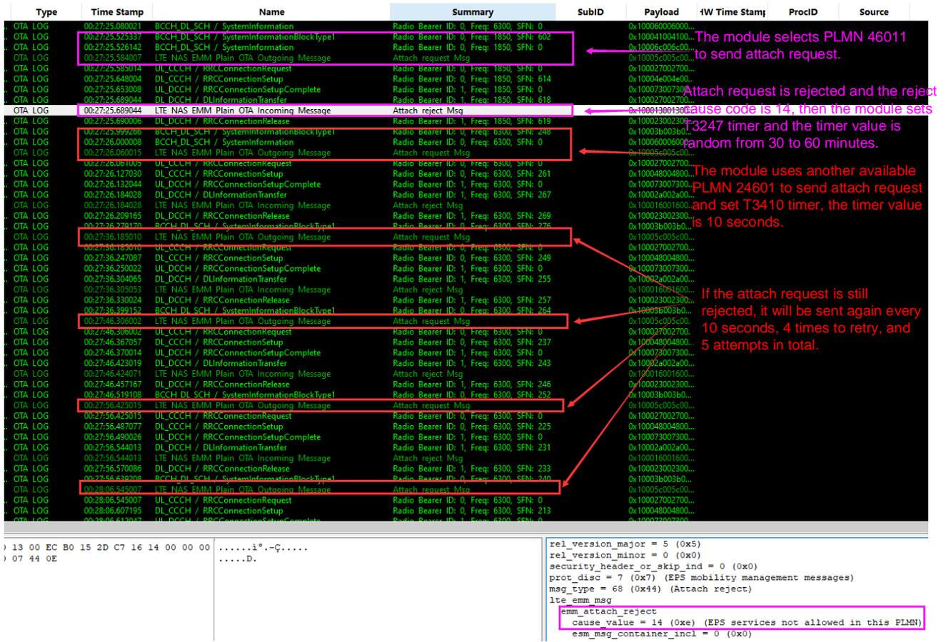
Figure 8: Module Received Reject Cause Code
